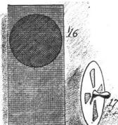
A disk of perforated cardboard or tin pivoted centrally to
