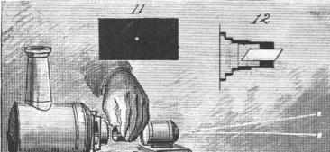
connected with the house water supply or it may be Upon this slide, which is also a piece of negative glass, used as a siphon, taking water from an elevated pail or tank. Only a small head is necessary to secure the desired results. The stream will be illuminated throughout its entire length, if a smooth flow of water is secured, and it may be tinted by inserting colored plates of glass in the slide receiver.
