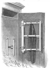
tical supporting strip, the rear edge of which is recessed and held to blocks at. tached to the door by screws. To the strip is hinged a rectangular frame consisting of vertical and horizontal pieces, the latter being provided with hooks on each side. Attached to the inner face of the outer strip by an elastic band or
