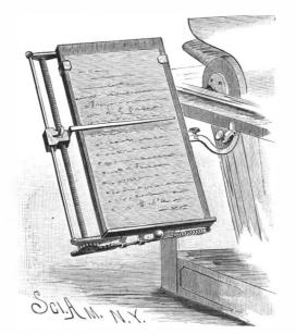
a clamp for holding the copy holder to the type writer. The hollow arm is so held to the bed as to permit of the edgewise adjustment of the latter.
