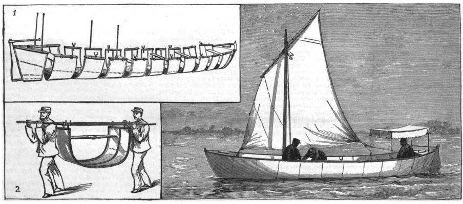
1. The twelve sections. 2. Carrying a section; weight, 75 pounds. 3. The boat afloat.
