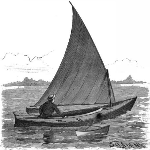
CLAPHAM'S LEE BOARD FOR SMALL VESSELS.
