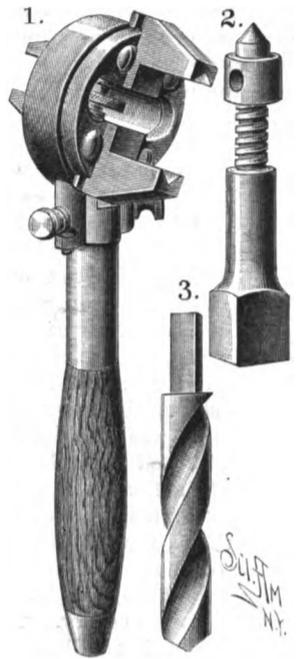
Screws passed through the socket, head piece, stems, and bar bind all the parts securely together. At opposite sides the socket is formed with bored lugs, in which are fitted pawls kept normally engaged with the ratchet teeth by springs. Into each of the pawls is fitted a pin, which passes through an L shaped slot in the lug. Either of the pawls can thus be withdrawn from the teeth of the disk, which can be turned in either direction.
