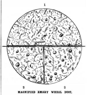
prevents the material being ground from being brought into contact with the cutting edges without undue pressure. The characteristics of a wheel of this kind are the rapid glazing of the surface and the slowness of its cutting.
