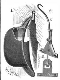
hook back into hook, A, is made of metal, and is hinged to a plate, B, attached to the sweat band inside of the hat by means of points stamped out of the plate. As represented in Fig. 2, the plate is with a holding lip under which the hook is adapted to be sprung for holding it turned
