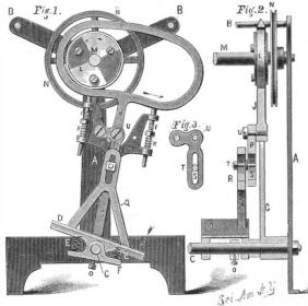
elbow lever, P. The upper arm of this lever is pivoted to one of the prongs of the fork, H, and the other arm is furnished with a longitudinal slot, S (Fig. 2), through which and the slot in the standard, Q, passes a pintle by which the pressure upon the wheel, L, can be regulated.
