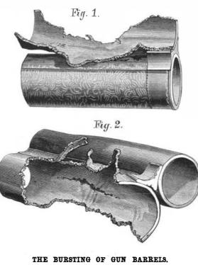
experiments have consisted in discharging guns which had been obstructed at the muzzle by all sorts of different substances, such as mud, sand, water, snow, stuck bullets, etc., and of whatever value the experiments may prove to be, they show one fact very conclusively-that it makes little odds whether a barrel be obstructed with a bullet or simply with wet sand; in either case the result may be
