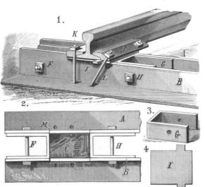
the ties, and the blocks or cushions can be taken out and renewed without disturbing either the ties or the rails. This invention has been patented by Mr. Charles H. Van Orden, of Catskill, N. Y.
