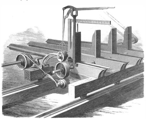
SCOFIELD'S STEAM LOG SETTING APPARATUS FOR SAW MILLS.
