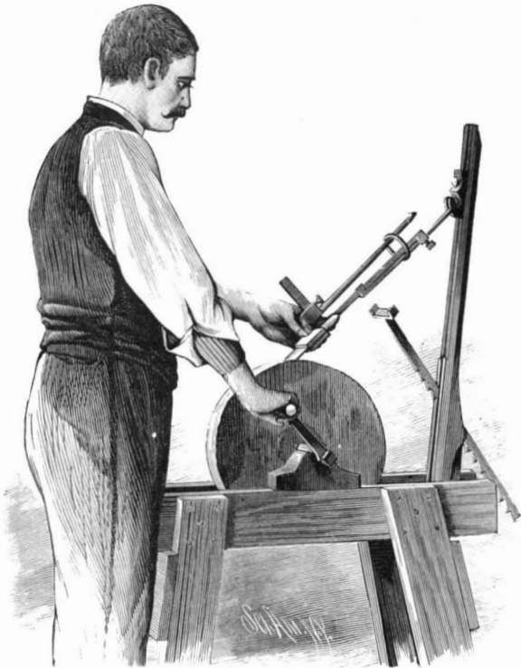
BAYHA'S TOOL HOLDER FOR GRINDSTONES.
