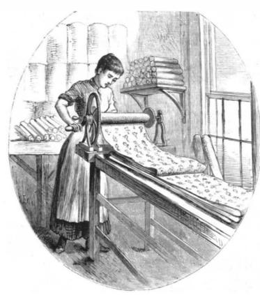
THE MANUFACTURE OF WALL PAPERS.-WINDING IT INTO ROLLS.
