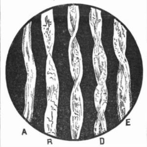
A. Glassy, structureless fiber.—B. Thin, pellucid, unripe fiber.—C. Half ripe fiber, with thin cell wall .- D and E. Fully mature and ripe fiber, with full twist and thick, well-defined cell wall.
