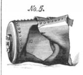
casting plainly embossed in the iron of the dome, which was crushed and detached from the boiler, as shown in sketch No. 5. At this point in its course it struck the curbstone, and several rivet heads were ground smoothly off as though by contact with a fast running dry grindstone, changing the iron to a blue color by the heat of the friction. Here also
