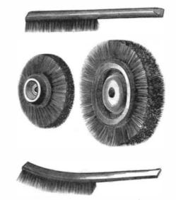
Where the article is to receive a deposit of gold or silver are usually made of brass or steel wire, and of a variety of its surface is usually softened by slightly amalgamating it shapes to suit the object. Some of the forms are shown in
