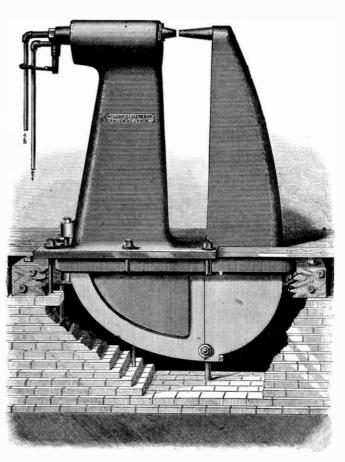
caused this, at all times equal, motion of the riveting die to the accumulator is shut off from the pump; the pump rewater directly into the accumulator.
