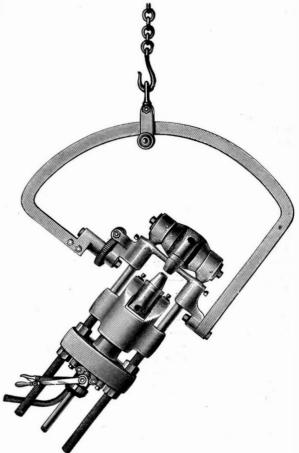
Fig. 3.-SUSPENDED RIVETING MACHINE-BOTTOM VIEW.
