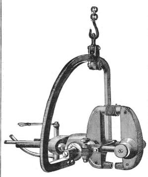
Fig. 1.—PORTABLE RIVETING MACHINE.
