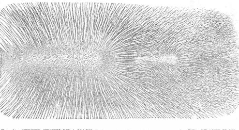
FIG. 29.-CURVES SHOWN BY A MAGNET ACTING INDUCTIVELY ON A CYLINDER OF SOFT IRON.
