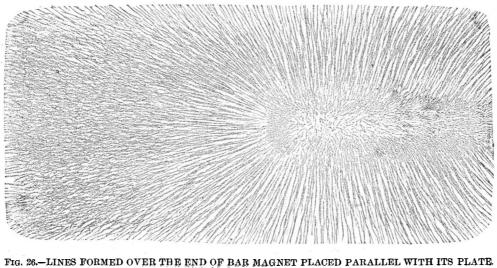
filings should remain unattached, they are removed from the plate by letting its edge fall squarely on the table.
