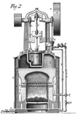
VERTICAL SECTION OF ENGINE AND BOILER.
