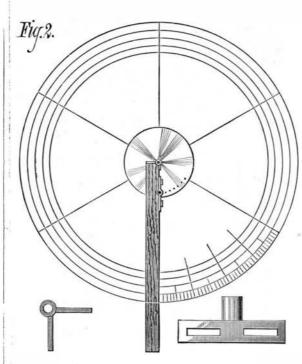
INDEX PLATES FOR GEAR CUTTING.
