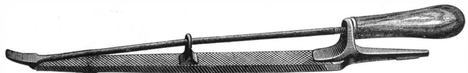
Fig. 29.—SURFACE AND FILE HOLDER.
