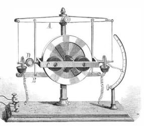
The instrument shown in the engraving should, when the axis of the frame, C, is adjusted equatorially, indicate 15° motion per hour in any latitude. The possible application of this instrument in a larger form to equatorial telescopes in place of the present clock trams, suggests itself. The only difficulty, if any, would be in providing telescope mountings of sufficient delicacy.
