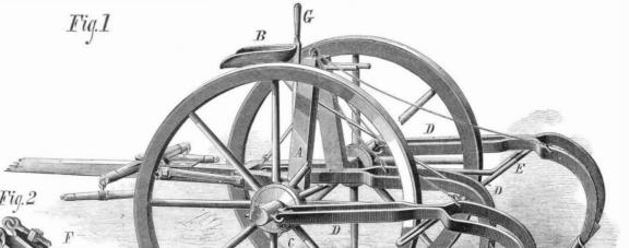
F, shown in Fig. 2 of the engraving, is attached to the axle by means of the middle pair of hook bolts. The wheel. F. is free to move up or down, by this arrangement each wheel will mark the ground distinctly, no matter how rough or uneven it may be. The implement is converted into a corn plow by removing the wheel, F, and moving the wheels from the
