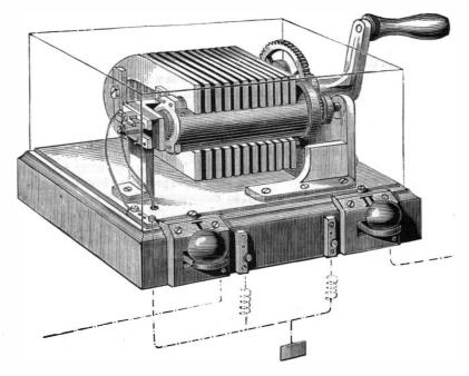
Fig. 3.—INSTRUMENT FOR TRANSMITTING ALARMS.
