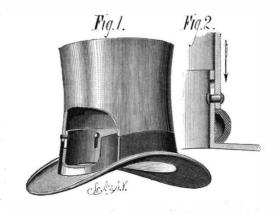
correct, even during the changes going on under the scouring fitted to the head. The body slides on the rim portion as shown in section, Fig. 2, and is guided by slots and pins, and supported by a cushioning spring. This device was patented through the Scientific American Patent Agency, February 26, 1878, by Mr. José M. de Celis, of New York
