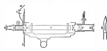
Fig. 1.—SACCHAROMETER IN SECTION.
