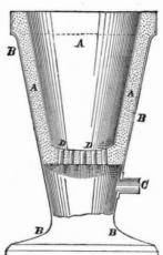
sketch of a simple little furnace, well suited for brazing, hardening, and tempering small taps, dies, drills, etc. A is an ordinary flower pot, having a number of small holes, D, drilled in the bottom. B is a frame or casing made of sheet metal, and C is a blast pipe, to be connected with a small blower. The plan might be still further cheapened by setting the flower pot bodily into another one of smaller size, the space between the bottoms then forming the chamber into
