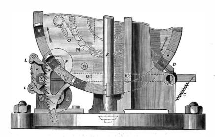
Fig. 5.-MECHANISM OF FIRE GONG.
