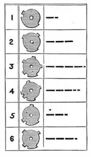
Fig. 2,—CONTACT WHEELS AND SIGNALS.
