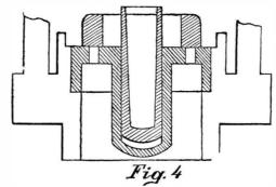
4. Double seated safety valves, of the same general form as the double puppet valve, the upper and lower parts being of different areas, so that they move easily and expose large areas of opening. The practical difficulties of construction, however, will probably prevent the adoption of this plan. The Committee report that they "can say nothing favorable of any of this construction that were tested."
