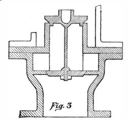
3. Annular safety valves, with two seats upon an annular opening (as shown in Fig. 4), with a view of obtaining a
