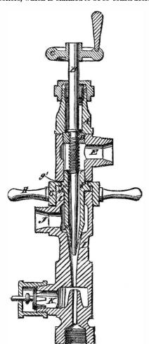
require any internal packing, as to prevent locking or bursting and side leakage, and as to work equally well at any pressure of steam. It may be detached, examined, and again attached in a few minutes without interfering with the working of the boiler.
