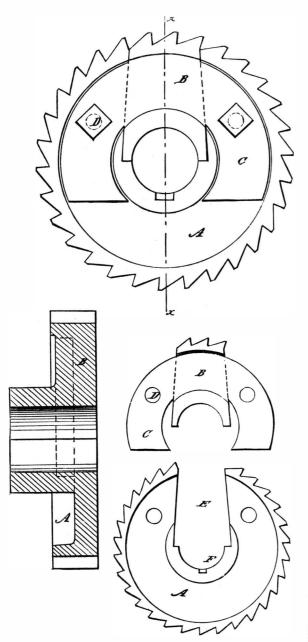
gether at the sides of the wheel. One part of the wheel may also be dovetailed in the other, to sustain the expanding action of the key better than in the common way.
