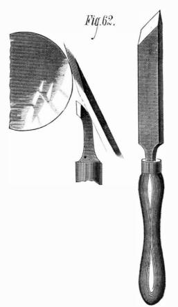
beveled at the cutting end on both sides (as shown in the edge view), being ground very keen. It is employed for fin-
