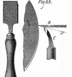
askew to the center line of its length. Furthermore, it is likely to rip into the work, and the position shown is all that is necessary, providing the cutting edge be kept properly sharpened. This chisel is also used on side faces
