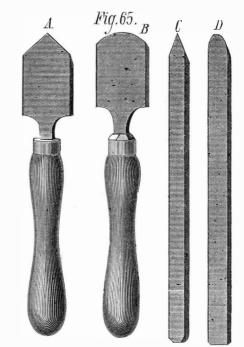
quence, it is less liable to cause the work to jar or tremble. It is usually made about 2 feet long, which enables the ope. rator to hold it very firmly and steadily. It is used with its top face lying horizontally, and should be kept keen. D, in
