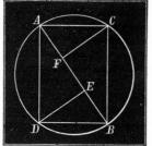
To cut the best beam from a log, divide the diameter, ab, into 3 equal parts, af, fe, and eb; and from e and f, draw the lines fc, ed, at right angles to ab. Join ac, rd, bc, and bd; then abcd is the cross section of the strongest beam.
