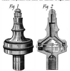
poor one will, the quantity of gas burnt being equal. 2 The intensity of the light increases with, but in a greater ratio than, the size of the slit. 3. The increase of illuminating power varies with the decrease of pressure. 4. The gas should be burnt at the lowest possible pressure. 5. The pressure should remain constant; and 6, the pipes should be large enough for the amount of gas carried through them.
