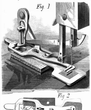
It is obvious that, in order to give a button the necessary movement under the needle so that the latter can pass backward and forward from hole to hole, a different feed motion from that usually found in sewing machines is needed. And, moreover, such motion must be adjustable according to the distance between the holes in the button. This seems to be neatly accomplished in the present device.
