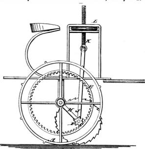
sired, or as the character of the land to be operated upon may require. To the center of the bail, attached to the saw shaft, is pivoted the end of a screw, K, which passes up through a hand nut, L, swiveled to a bracket, attached to the frame, so that, by turning the said hand nut, the saws may be adjusted te enter the ground to any desired depth, or may be raised from the ground. The axle is suitably bent to accommodate the saws.
