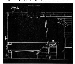
but this should only be done in the case of very short tubular boilers, and the roller support is preferable for every case. Very long boilers require to be supported at intermediate points. This is commonly done by means of suspension rods, which can be adjusted by nuts, but this practice is by no means commendable. When a fire is made under a long boiler, the bottom becomes more highly heated than the up per portion, so that the boiler tends to take a curved form
