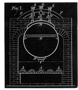
through the tubes or flues to the front connection, A, and thence pass to the chimney by the flue, E. The engraving shows one of the best arrangements of fronts for this kind of boiler.
