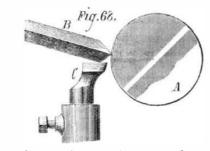
hand rest (the point being used to cut, as shown in Fig. 68, A being the work, B, the graver, and C, the lathe rest), it turns very true and cuts easily and freely. This, therefore, is the position in which it is held to rough out the work.
