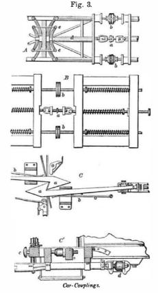
respective point-headed hooks come in collision. The springs, b, keep the hooks together when connected. The lower view C', exhibits also the spring buffers, c, above the hooks, which act as fenders to the cars and deaden the blow as the cars strike against each other when the speed of the train is checked. The coupling hooks have, besides, springs, d, for the same purpose.
