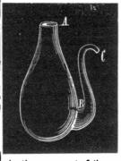
oils? A. A Flor conical in form, and at the side is a spout, B C, com municating with the bottom, the orifice, C, of the spout being much lower than the mouth, A, of the receiver. The distilled product being poured into this vessel, the oil separates from the water, and occu-
