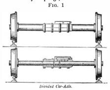
In Figs. 1 and 2 are represented two forms of divided car axle. When the axle is constructed of a single piece of metal, with the wheels fixed firmly thereon, it is subject to severe torsional strain in turning curves. The outer wheel has a larger circle to traverse, thus compelling the wheel on the inner and shorter circle to slip. This torsion of the axle
