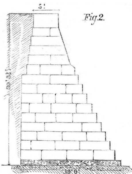
on a bed of concrete and riprap. The height is 30 feet 3 1/2 inches. Behind this wall, however, is merely earth thrown in and not packed or rammed down,—a precaution, in fact, not as yet taken, because no craft larger than a ship's launch was expected to come near the work. The consequence was that the loose soil yielded, while the ship escaped with no other injury than some scratches and a lump of granite imbedded in her bow.
