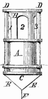
head of B must be ground to a perfect joint, and may be supplied with a flexible gasket to prevent all leakage. As C passes freely back and forth through A, the valve can never get foul or fast in it, as has so often been the case, causing many disasters. The dotted lines represent the apex of the balloon. A glance will show any scientist how the valve can be secured in position. The whole apparatus may be made of any suitable metal or of vulcanized rubber.
