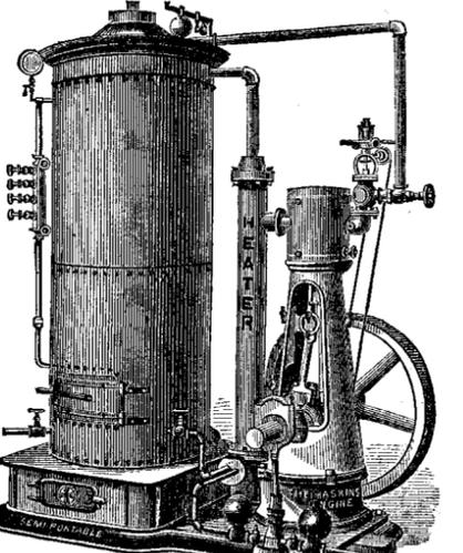
(10 HORSE-POWER.) Our Combined Engines and Boilers are made in quantities and to standard gauges, so that all parts are interchangeable.
