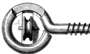
In the inner side of the eye a groove is formed. The pulley revolves on an axle the ends of which are made in segments of circles, A, the circumferences of which fit into the groove in the eye. By this construction the pulley may be turned in any desired direction by moving the ends of its axle. The screw eye may also be turned in its support, so that the cord passing around the wheel may be led as required. Patented, February 11, 1873, by Mr. Charles C. Moore, of New York city.
