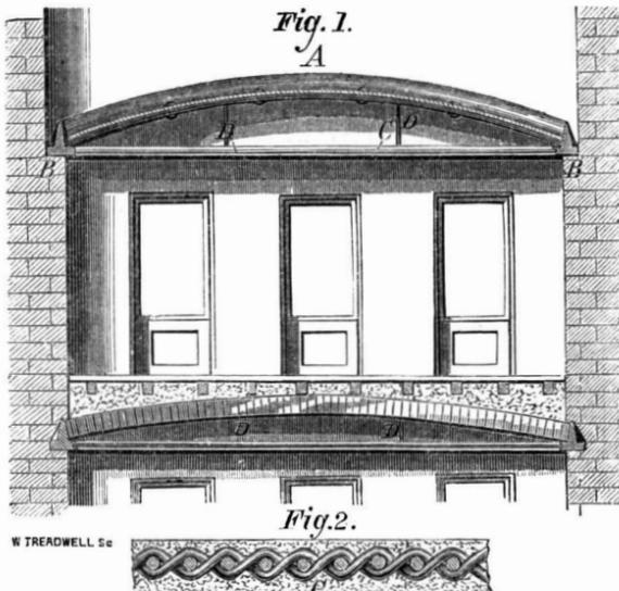
short rods, D, from above, and upon it the plaster is applied in the ordinary manner. The device is necessarily fireproof, and is said to form firm floors, incapable of transmitting sound to any considerable extent. Patented through the Scientific American Patent Agency, April 1, 1873.
