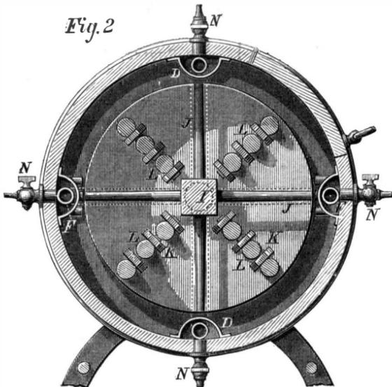
condensation. When feathers, hair, and like substances are to be acted upon, the bars, L, are removed, and the beaters, J, placed in position. The material is then packed in the cylinder, and the subsequent operation is the same as above described. It is proposed to construct the machine in sections so that it can be readily taken apart and packed for transportation.
