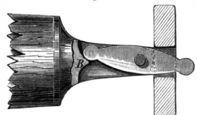
The trace can then be easily slipped on, and the button returned to a vertical position. The stub is tapered so as to cause the trace to slide against the button, and is made thicker at the point where the latter is pivoted to ensure the requisites strength. Patented October 1, 1872, by Mr. William C. Shepherd, of Cleveland, Ohio.
