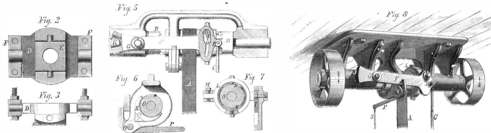
or horizontal beds. The present improvement embodies the peculiar advantages of both styles. The arcs, B, are firmly held by the bolts, C, so that the bed may set inclined for work in which the punched pieces are desired to slide out by their own gravity, or adjusted to the horizontal position.
