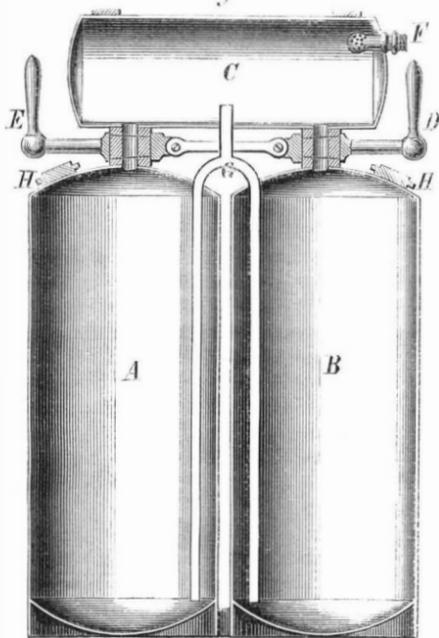
handles being joined by a rod so that either hand may be used for operating them, hose coupling, F, equalizing pipe, G, which keeps the pressure uniform throughout the machine, and stoppers, H, which are removed for charging the machine.
