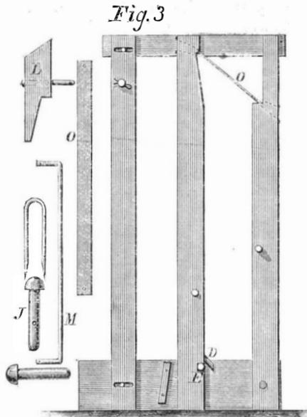
arrangement of the closing and latching devices, the device for adjusting the space for the animal's neck, and enlarged views of the arms, hook, button, etc.
