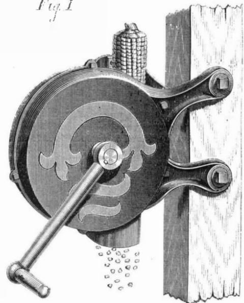
remains. B is a disk, having, about midway between its center and circumference, a circle of cogs which mesh into the pinion of the fluted roller. This roller, with its pinion, is cast all in one piece. Suitable bearings for it are bolted to the case, as shown.
