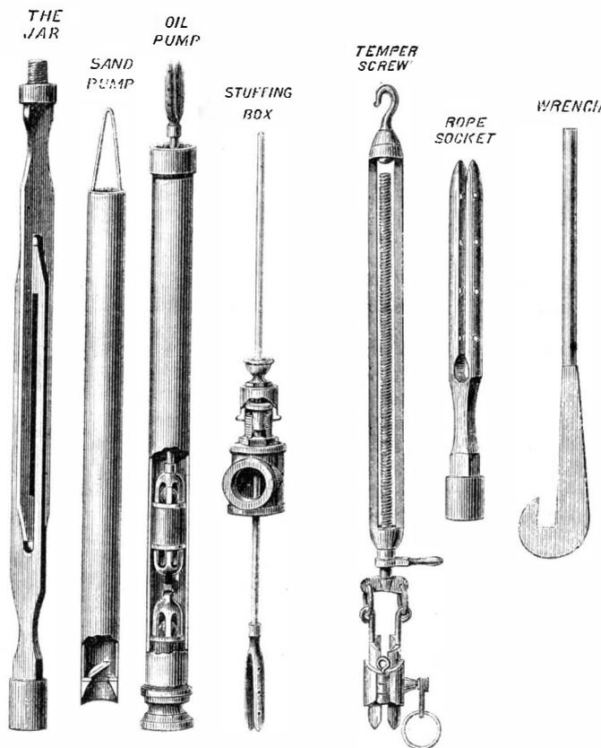
in boring for oil in Pennsylvania is extracted from Blake's "Notices of Mining Machinery":
