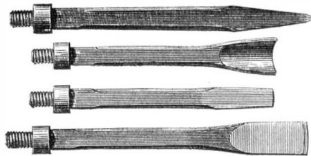
The bits are represented by the annexed cuts. They are 3 $\frac{1}{2}$  inches broad on the face, and the reamers are 4 $\frac{1}{2}$  inches. They are made, however, of various sizes, and all have strong, square shanks, so that they may be firmly screwed into the auger stem, made of 2 $\frac{1}{2}$  inch iron and 20 feet long.
