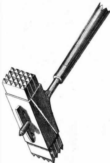
end of the handle, which projects through the clamp. The handle passes through four four-pointed chisels, as shown,
