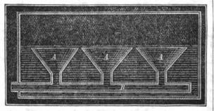
Annexed is a sketch of another device for the same purpose from a rejected application filed by G. Ortleib, in 1852. It consists of a series of funnel-shaped vessels, a a, connected at their bottoms to a horizontal tube, b, having at its outer end a blow-off cock. The tops of these vessels reach to near the top of the water, and the scum settles in them and is
