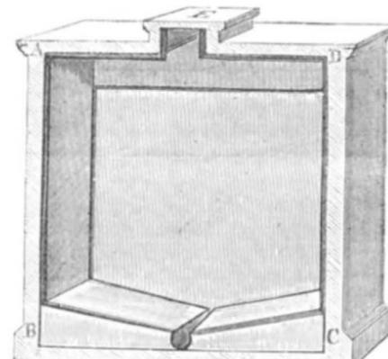
An air-tight lid is hinged to the top of the safe, so packed as to prevent egress of vapor, and easily opened and closed.
