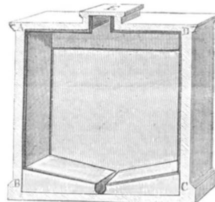
An air-tight lid is hinged to the top of the safe, so packed as to prevent egress of vapor, and easily opened and closed.
