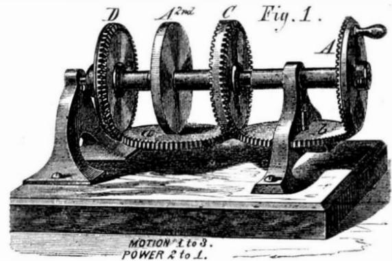
verse by the action of b, a would make a second revolution upon its own center, which would be communicated to D, making three, viz.: one by the pin or bodily motion of a, one by the inertia of C, and one by the reverse of C, making three, which may be decreased or increased as desired, this being the unit of the machine and its simplest form.
