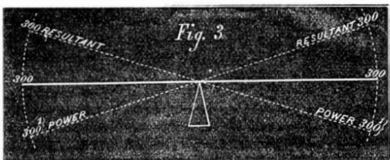
The same remarks are plainly true here. The 300 on each end of the lever are not the cause of motion, but are the cause of balance or rest; and any excess on either end makes them alternately the power and resultant.
