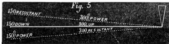
And that the center and end become alternately power and resultant, as excess is placed upon either.
