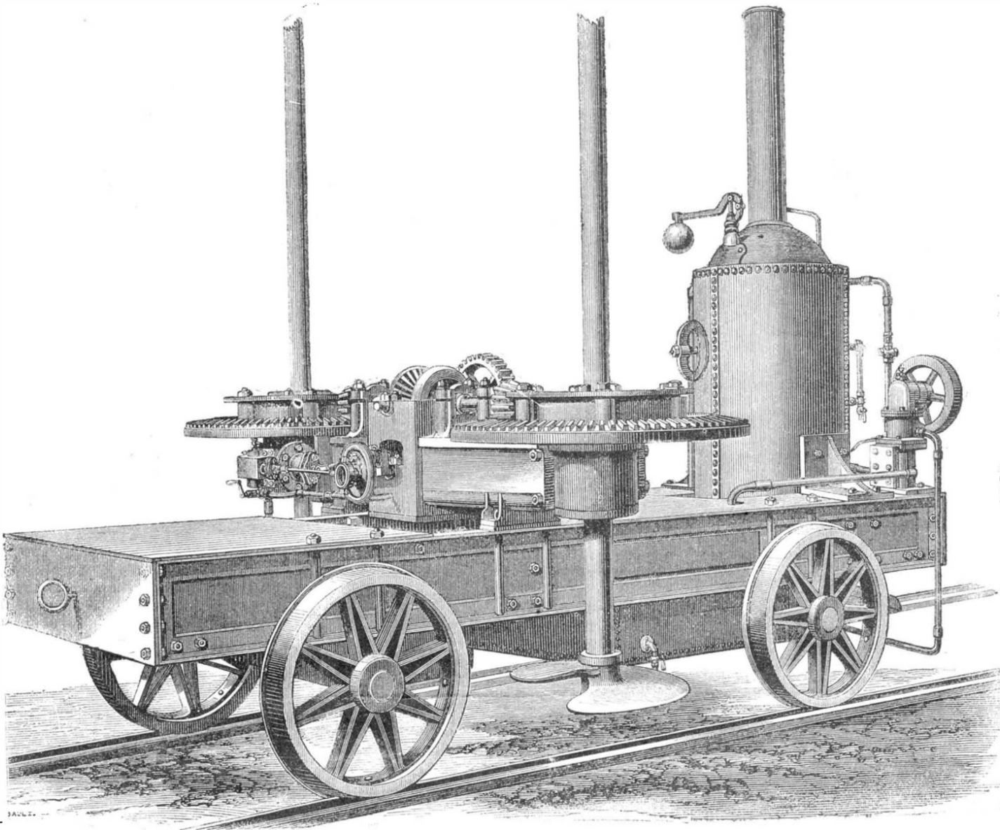
APPARATUS FOR SINKING SCREW PILES BY STEAM.
