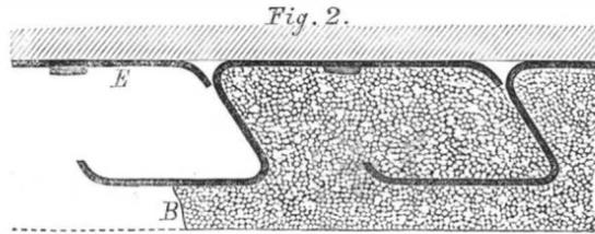
In this engraving the joists are lettered A; B is the concrete; C the lath and plaster, or ceiling, on the under side of
