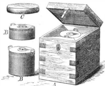
A is the box, lined with felt; B B the saucepans fitting into the box; C the felt cover, to be placed on the top of the saucepans.
