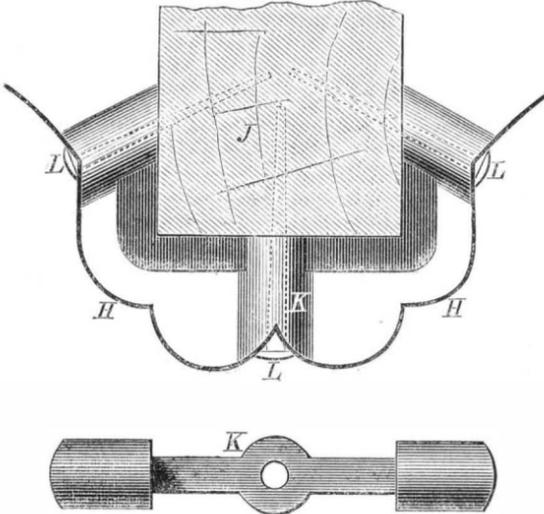
Fig. 2 is a section of the iron laths and the plastering, showing the peculiar form of the laths and the manner in which they support the plastering.
