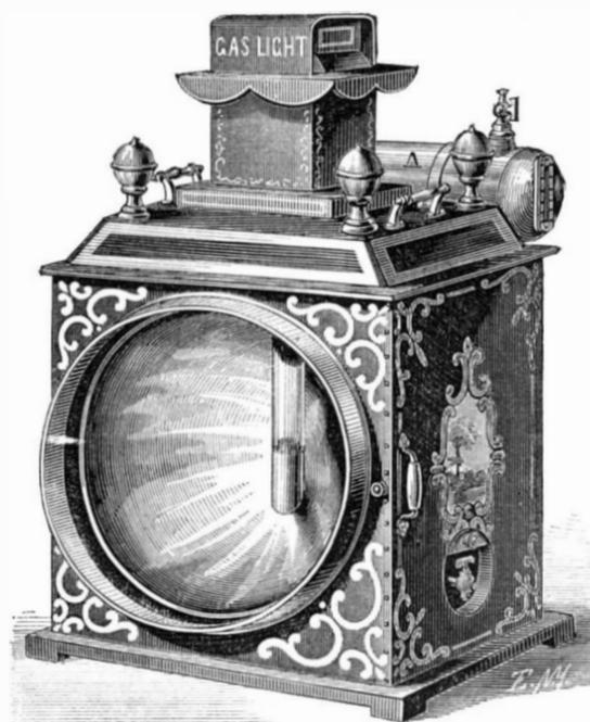
the boiler of the locomotive on the opposite side of the case, circulates around the vaporizing chamber, converting the liquid into vapor, and passing up from the heater the hot air is injected, and the gas flows through the burner. The pipes
