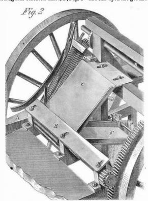
From the incline, C, the ears pass to a pair of horizontal rollers under the cap, E, by which they are husked, when they drop on the platform, F, Fig. 2, and are delivered into bags, or other suitable receptacles at the rear, the husks, as they leave the rollers, dropping to the ground, or, if desirable to save them, to any proper receptacle under the machine.
