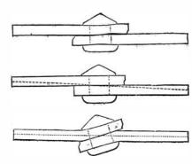
and thereby adds to the tension; and the lap of the sheet throws it out of the line of the tension exerted by the pressure of the steam, the tendency being to bend the sheet as shown in the cut.
