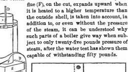
It has been found by actual experiment that single riveted seams have but fifty seven hundreds of the strength of the weakness is greater than the proportion of the iron, cut which they would resist compression at the same temperature
