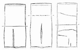
inches diameter, to the same ordeal of heating and partial cooling; one of steel, one of wrought iron, and one of cast iron. The cylinders were ruptured in the manner shown, Each became longer—the dotted lines on the cuts show the original length—the central part of the metal being squeezed out to greater length by the contraction of the outside, which cooled first, and contracted upon the interior metal, like the tire upon a wagon wheel.
