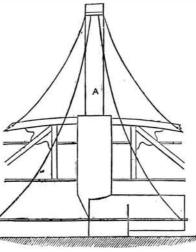
plosion is more common than the rupture of steam chimneys on the kind of boilers almost universally used on river and sound boats along the Atlantic coast such as shown in the cut. I do not believe a single case can be remembered in which a steam chimney has been ruptured longitudinally. I have known of a
