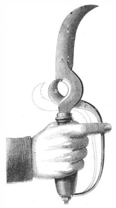
curved as at A, similar to the blade of a pruning knife. Its back at the rear end next the handle is formed into a curved edged jaw, in connection with which the spring jaw, B, completes a device for stripping the cane of its leaves.
