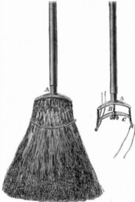
inventive genius of the country has designed several devices for securing new corn to the handle when the original is worn out, with but little labor and diminished cost when compared with the original first price of a broom. The one shown in the engraving is exceedingly simple and very cheap.
