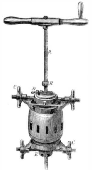
termines the taper of the hole to be bored. E is an open nut by which the cutters can be drawn back to the butt of the hub without turning the handle or shank.
