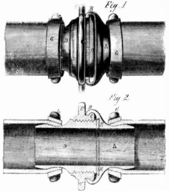
of the coupling. This collar is connected with the part, D, by a left hand thread on its inner surface, engaging with a corresponding thread on the outside of the part, D. A recess inside the head, B, receives an annular packing of leather or other suitable material, seen in section at E. The collar, C, is provided with snugs, F, by which it is turned, either with the hand or a common hose wrench. The force of the hand, however, is in all cases sufficient to make a perfect joint.
