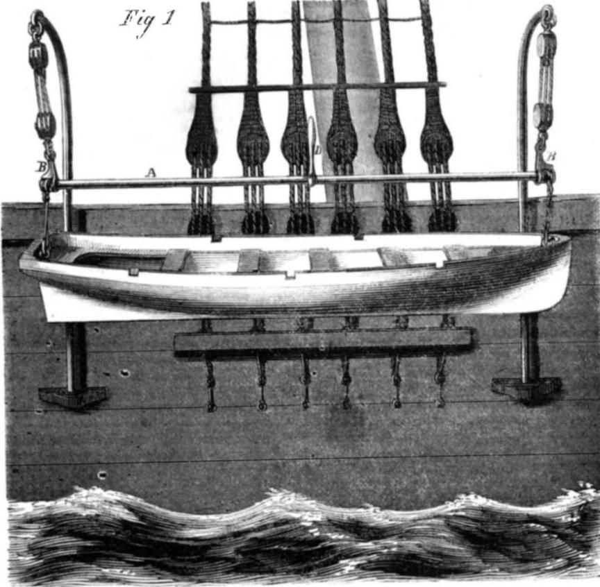
Now it will be seen that the loops resting, as at E, in a score nearly at the end of the bar, a partial turn of the handle, D, will throw them off, both at the same instant. Either the bar in the boat passing under the thwart or that one suspended to the fall can be used, the operation in both cases being the same. The bar can be secured by any simple means so that it may not be tampered with.
