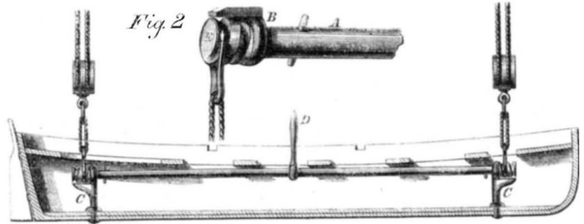
MASSEY'S BOAT-DETACHING APPARATUS.
