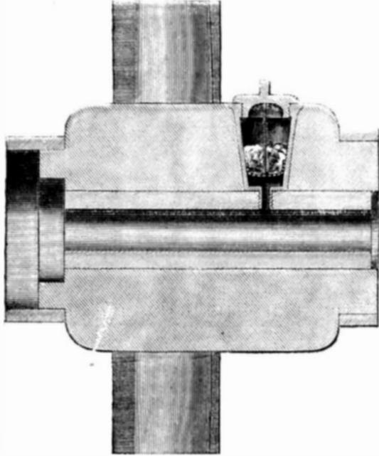
filled with oil the sponge prevents it from running out of the little pipe at the bottom when the carriage is at rest. When in motion the jars and jolts serve to squeeze the sponge and allow the escape of the oil to the axle. The vehicle may be run for weeks with once filling the reservoir. The only projecting part is the cap, which is ornamental and stands but slightly above the hub.
