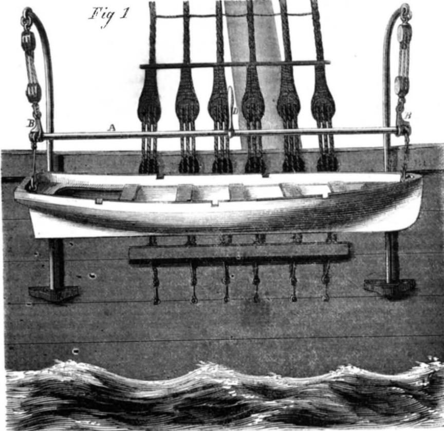
We give two engravings which represent two arrangements of the same plan for securing the safe launching of boats from ships under circumstances of danger. Fig. 1 shows a boat suspended at the davits ready for lowering, and Fig. 2 the section of a boat with the apparatus secured to its bottom inside, and a view, enlarged, of the disconnecting bar. This bar, in which the principle of the device is mainly located, is simply a bar, A, of metal, of a proper length for the boat,
