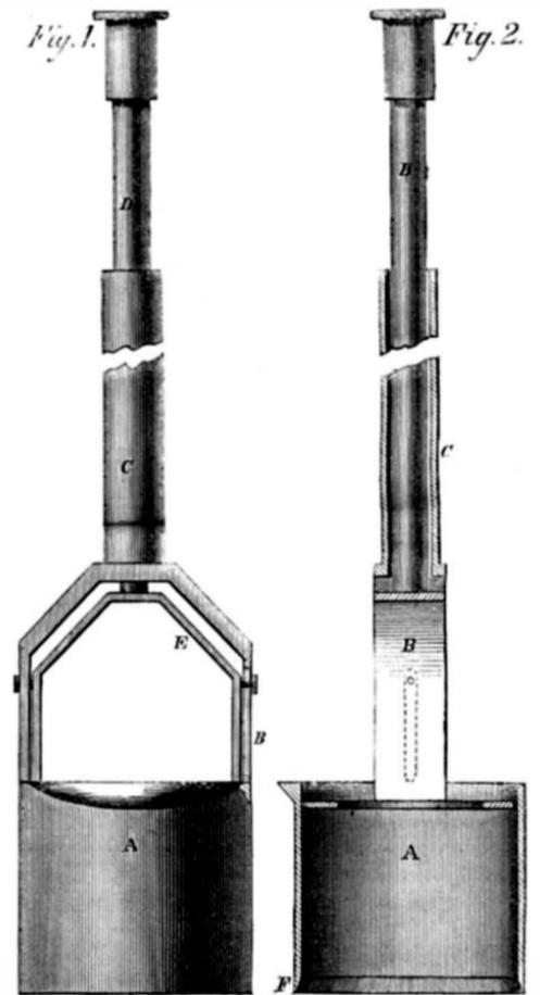
From two opposite sides of this cylinder, at the top, rise the arms, B, which are fastened to the hollow handle, C. Inside this hollow handle is a rod, D, terminating at the top in a knob, and at the bottom secured by the yoke, E, to a ring loosely fitting the interior of the cylinder. The upward and downward movement of this ring is guided and governed by pins sliding in vertical slots in the upright portion of the arms, B.
