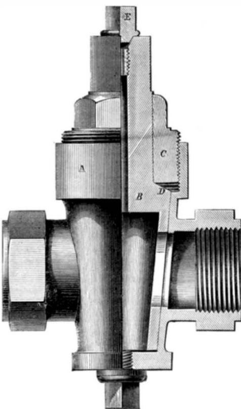
ded the attention of engineers and others engaged in steam and gas work. The objects sought were a straight port or way, which is not secured in the ordinary globe valve; perfect joints without the possibility of leaking; freedom from danger under pressure, and security against freezing. These appear to have been attained in the cock shown in the en-
