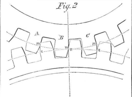
radius upon the pitch line, as in the figure, and taking half the arc thus subtended. The point, o', at the middle of this chord, is the center, and half the
