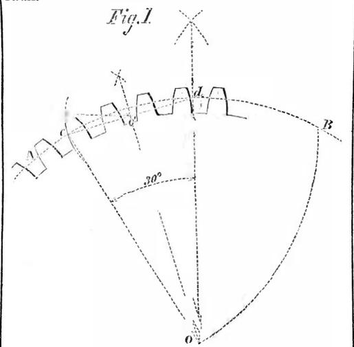
In Fig. 1, A B is a portion of the pitch line of a gear of which O is the center; c d is the chord of an angle of 30°, easily found by first stepping off the
