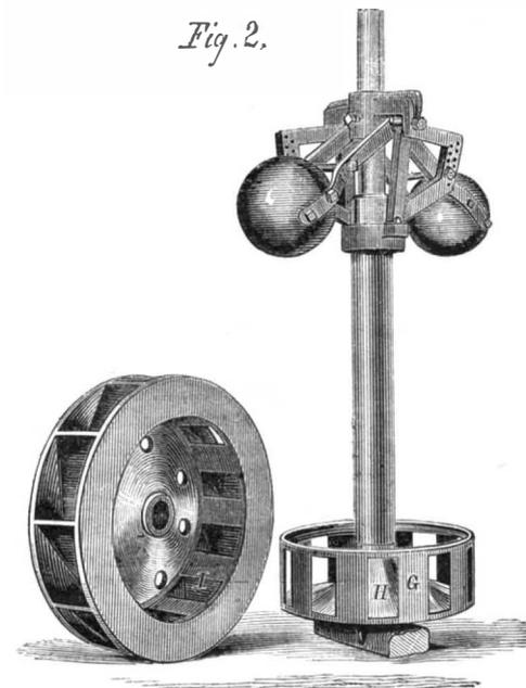
the end of a bell crank, D. The other end of the same connects with a collar on a cast-iron sleeve, E, fitting over the main shaft, and the governor levers also connect with it through the medium of a bolt, F. The sleeve, E, connects at the bottom of a regulator valve, G, Fig. 2.
