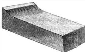
Fig. 9. A scraper tool with a slightly raised or concave front edge. Such tools cannot be used for brass as they are too sharp; the edges jump into the metal and spoil the work.
