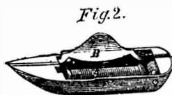
B, which causes the thread to be drawn from every part of the bobbin with equal draft. There is a screw on the top of the shuttle, by which the pressure of the spring on the plate, B, can be adjusted if necessary.
