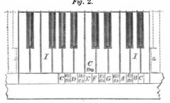
The fixed scale is shown in Fig. 2, lettered C C, D D D E, &c., corresponding with the denominations of the notes of a complete octave, the several
