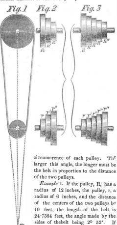
this angle is neglected, the length of the belt would be only 24.71 feet, making a difference of about one-third of an inch. If the pulleys are at 7 feet distance only, the length of the belt is 18.7479 the angle between the sides of the belt being 4° 5′ 46″. With neglecting this angle, the length of the belt is 18.71 feet, making a difference of nearly one-half an inch on a shorter belt.
