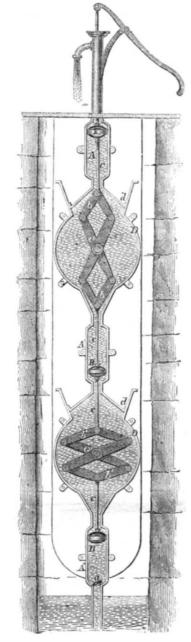
water from the well is drawn up. When B is depressed, it passes through the water in A by its clack valve being opened, and compressing the rods, b C, elevates the piston, B', thus bringing up more water, and at the same time the opening of the cross-rods and links, b' and C', depresses the piston, B," and the weight of water closes a.
