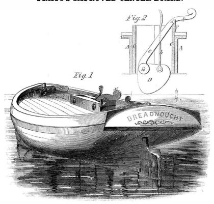
enabled to sail closer on a wind, and hence be | sailing on a wind. H is the handle or tiller much more under control and enabled to be kept from a lee shore. The oblique direction of D must be changed every time the vessel is in stays. As an auxilliary to D, the cutwater, G, is made to project from the vessel and to be movable like a rudder, that it may
