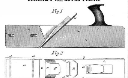
The stock of this plane is formed of wood with metal sides, and the front part is made adjustable by means of set screws, so that the "throat" may be enlarged and contracted at pleasure, as the nature of the work may require. Its construction will be fully understood by the following description and the accompanying engraving, in which Fig. 1 is a longitudinal vertical section and Fig. 2 is a plan or top view of the plane.
