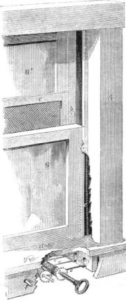
Our engraving represents a device invented by Wm. Huey, of Christiana, Pa., and patented by him Feb. 15, 1859, for the purpose of easily elevating window sashes and retaining them at any desired points in the frames.
