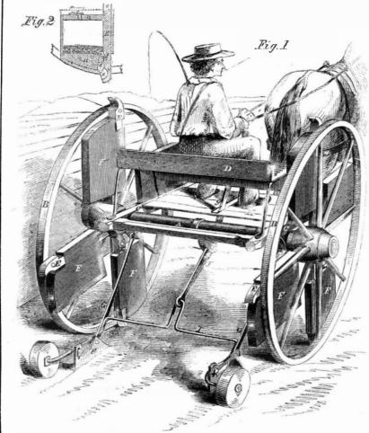
or fall in register with the recesses, e, in the bars, E, and the seed will be discharged into the holes in the earth made to receive it. by the projecting or outer ends of bars, E. The recesses, f, as the seed is discharged from the recesses, e, are filling with seed to be discharged at the succeeding revolution of the wheels. The shares, H, cover the seed; they may be elevated at any time by operating the front of the lever, which may be retained by any suitable catch or device.
